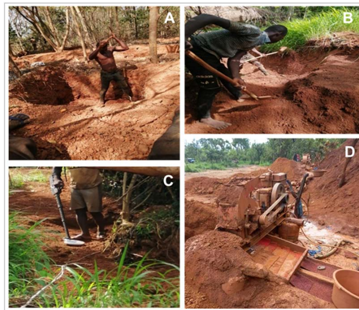
Figure 2. Main stages of gold extraction at Kouassi-Diètèkro and Kongoti: (A) Hole dug during the sinking phase, (B) Sand extraction and spreading, (C) Testing with metal detector for gold recovery, (D) Machine washing the sand
