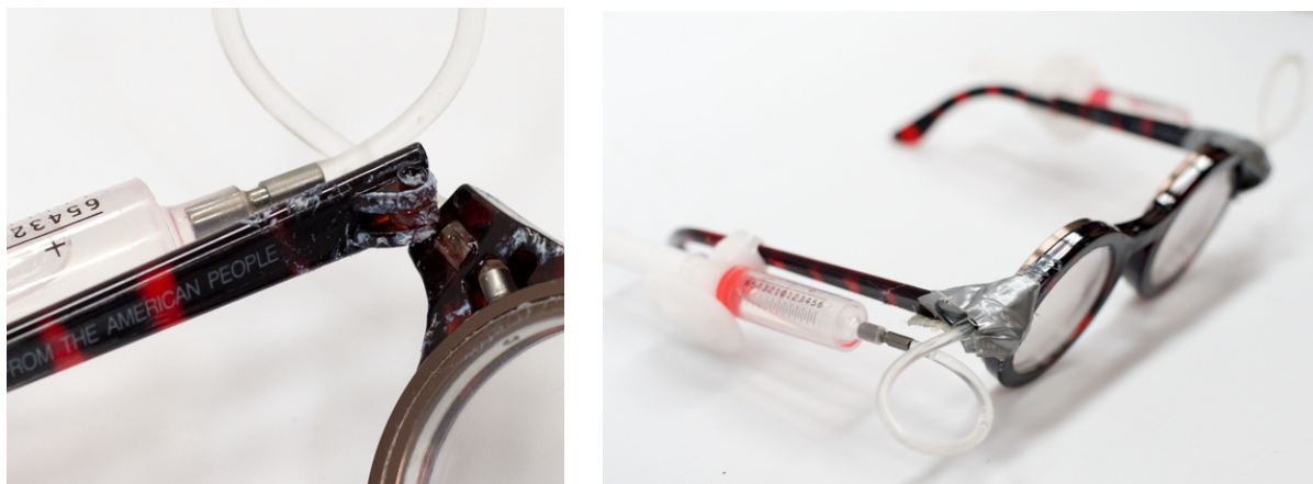
Figure 3. a) Detail of hinge break on an Adspec lens and b) the Adspec system fixed with duct tape.
