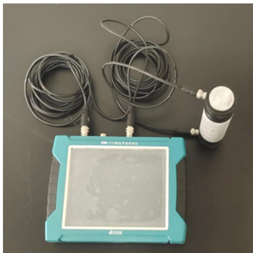
Figure 2. Ultrasonic testing equipment
