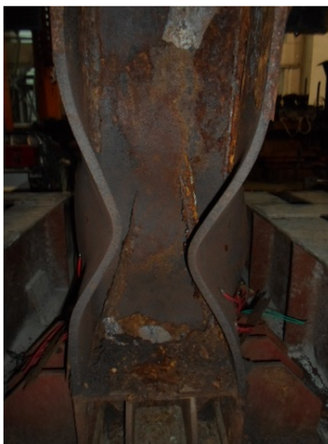
Figure 17. Comparison of failure modes between experimental tests and finite element simulations: (a) column 10; (b) column 1; and (c) column 2
