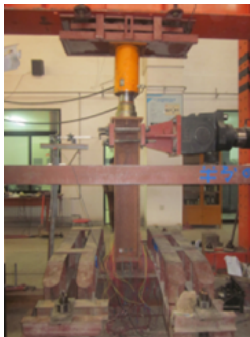
Figure 5. Actual test loading device
