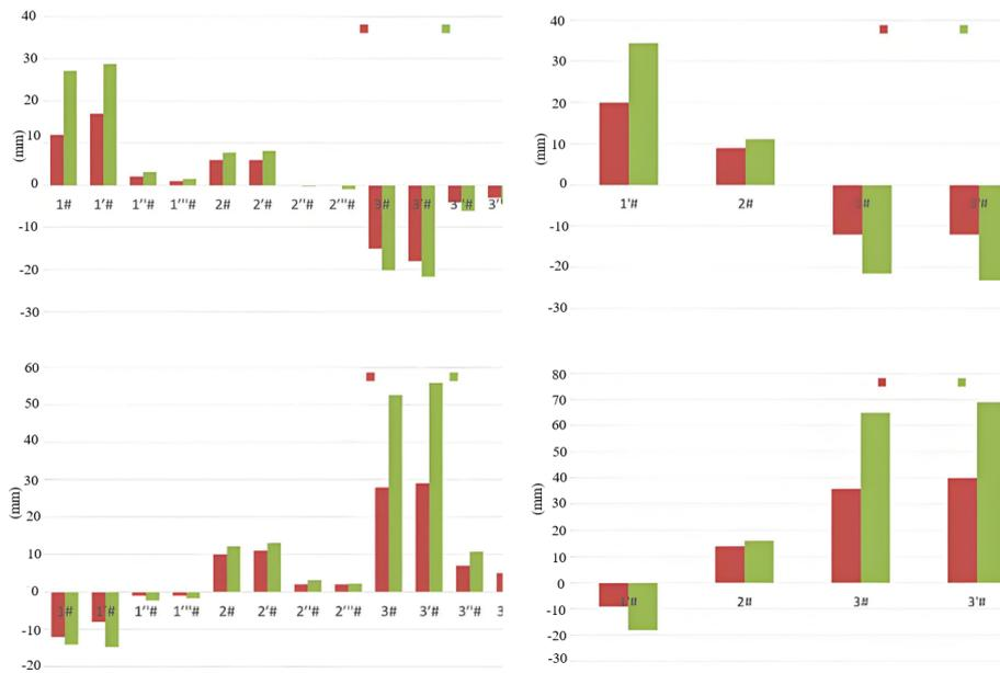
**Figure 10.** Comparison between measured and theoretical deflection values under maximum loading conditions for conditions 1 through 4
