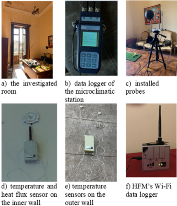
Figure 4. Equipment and sensors used for the survey
