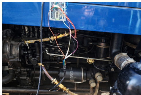
Figure 4. Integration of ESP32 and dual YF-S401 flow sensors for real-time fuel
