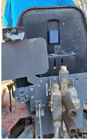
Figure 3. Installation of the MPU6050 IMU module behind the operator's seat for real-time velocity and slip ratio measurement
