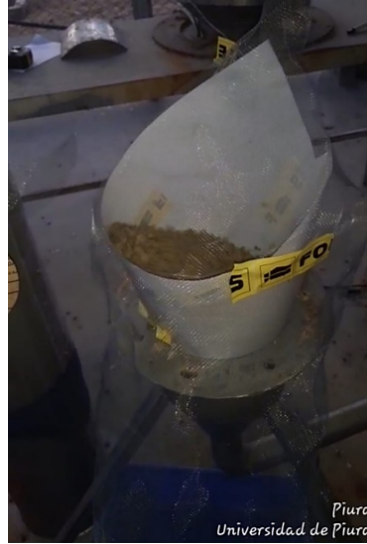
Figure 5. Fluidization test in a wider conical structure, showing improved grain motion for the 5 kg coffee mass
