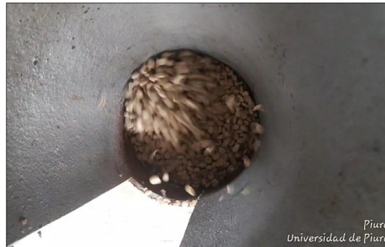
Figure 12. Fluidization behavior of 3 kg of parchment coffee in the cylindrical reactor at 60 Hz
