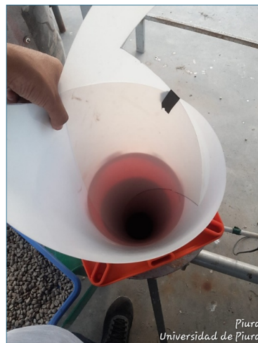
Figure 4. Fluidization test in a narrow conical structure, showing limitations when the 5 kg coffee mass becomes compressed
