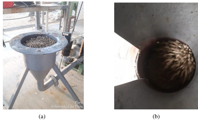
Figure 3. Preliminary conical-structure test: (a) distributor used in the prototype; (b) top view of the induced grain motion
