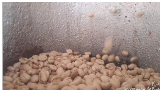
Figure 11. Fluidization behavior of 500 g of parchment coffee in the cylindrical reactor, showing localized rather than uniform grain motion
