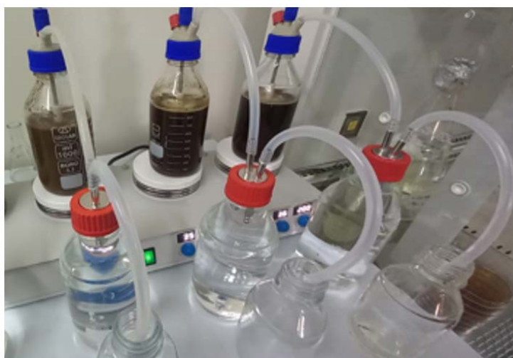
Figure 1. Experimental setup for biogas production
