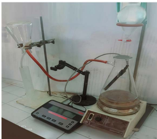
Figure 2. Experimental setup for pH monitoring
