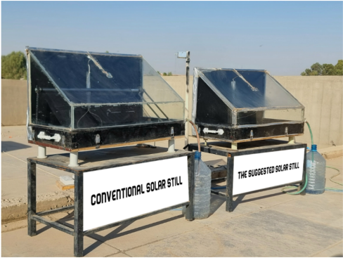
Figure 2. The conventional solar still (left) and the modified solar still (right) used to evaluate performance improvements in freshwater production under identical environmental conditions
