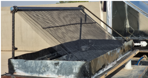
Figure 3. Mesh cotton inside the improved solar distiller
