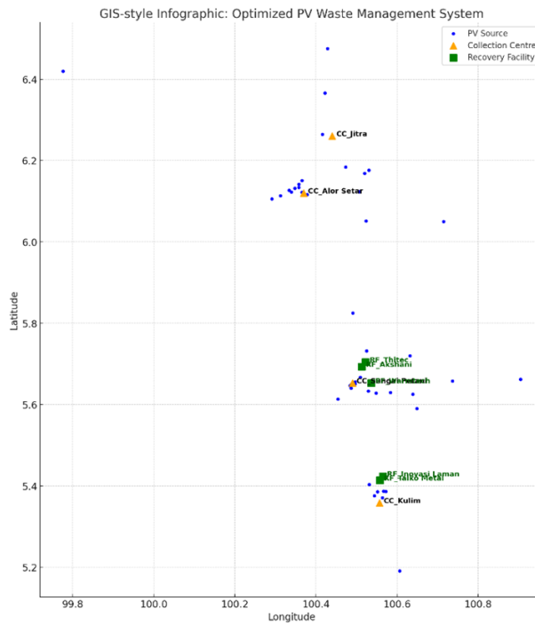
Figure 13. Geographic information systems-style infographic of optimized photovoltaic waste management system layout in Kedah
