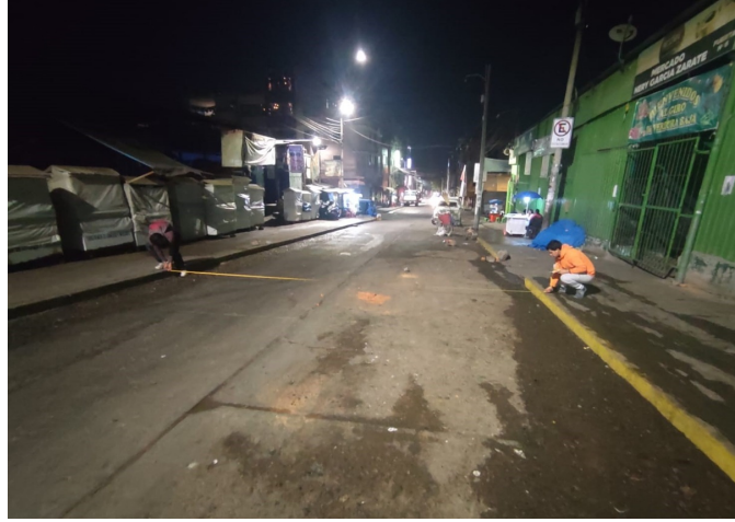
Figure 5. Measurement of roadways within the study area
