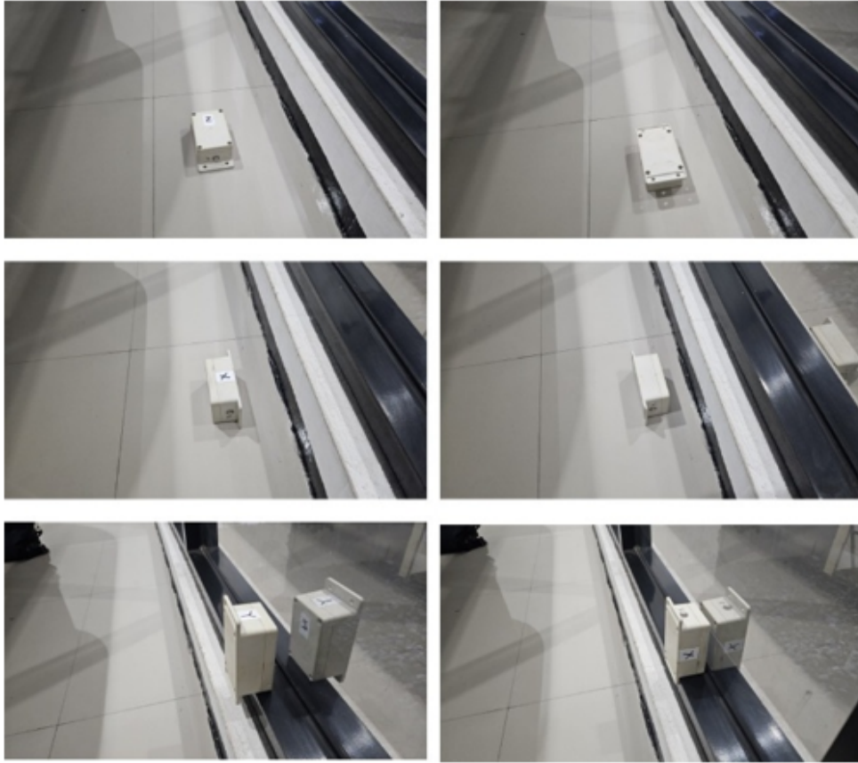
Figure 2. Six standard positions of the IMU tool for calibration measurement
