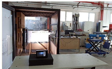
Figure 1. The experimental setup for Hailstone impact
