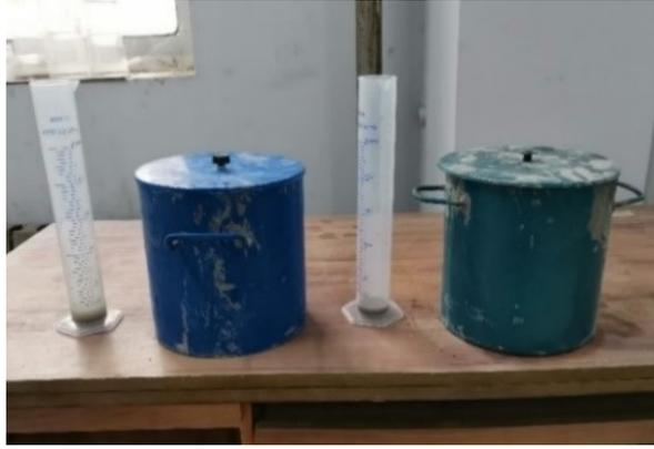
**Figure 5.** Test diagram of bleeding rate of fresh cement-based composite
