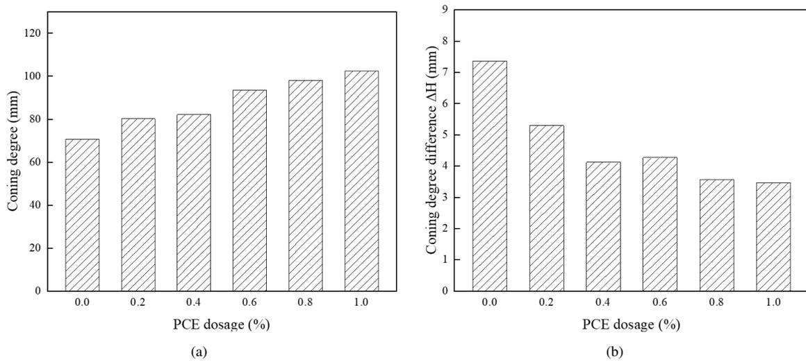
**Figure 12.** Effects of PCE Dosage on coning degree of fresh cement-based composites (a) Effect of different PCE dosages on coning degree (b) Effect of different PCE dosages on coning degree difference  $\Delta H$
