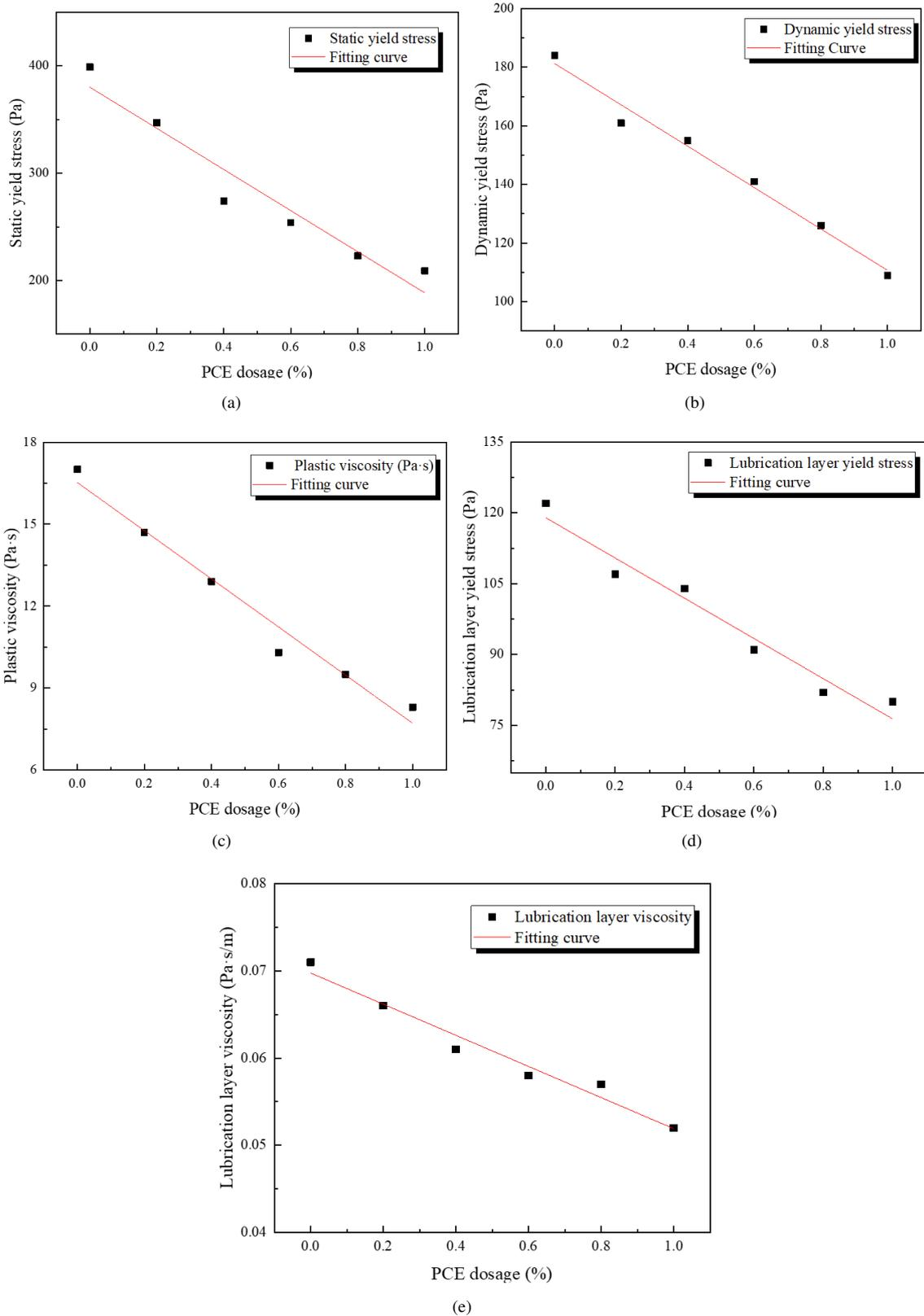
**Figure 9.** Correlation between PCE dosage and rheological parameters of fresh cement-based composites (a) Fitting curve between PCE dosage and static yield stress (b) Fitting curve between PCE dosage and dynamic yield stress (c) Fitting curve between PCE dosage and plastic viscosity (d) Fitting curve between PCE dosage and lubrication layer yield stress (e) Fitting curve between PCE dosage and lubrication layer viscosity
