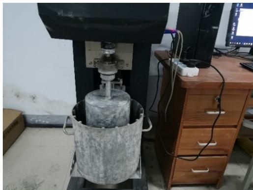
**Figure 3.** Field diagram of rheological test of fresh cement-based composites lubrication layer
