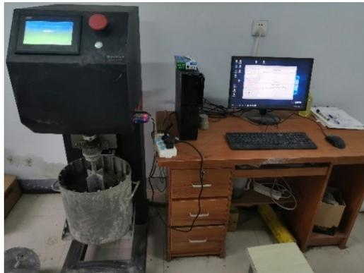
**Figure 2.** Field diagram of rheological test of fresh cement-based composites
