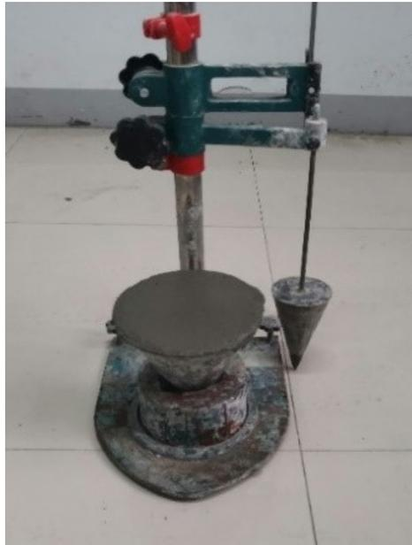
**Figure 6.** On-site photo of consistency test of fresh cement-based composites
