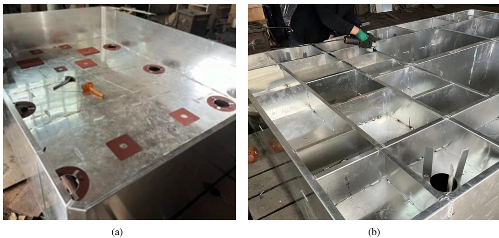
Figure 3. Platform main body model processing: (a) Platform main body bottom plate, outer wall, and internal equipment weighting; (b) Platform internal bulkhead
