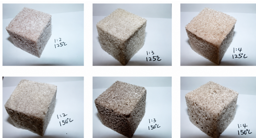
Figure 9. Bio-polyurethane foams from sugarcane bagasse by microwave liquefaction [188]
