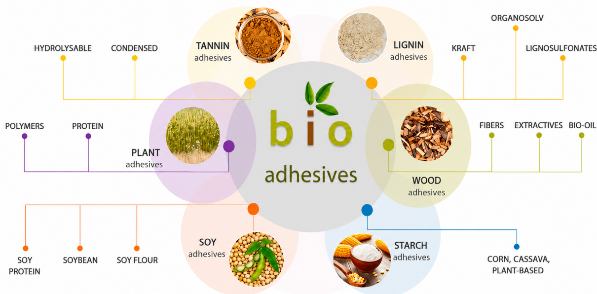
Figure 8. Bio-alternatives for the production of wood bio-adhesives [177]
