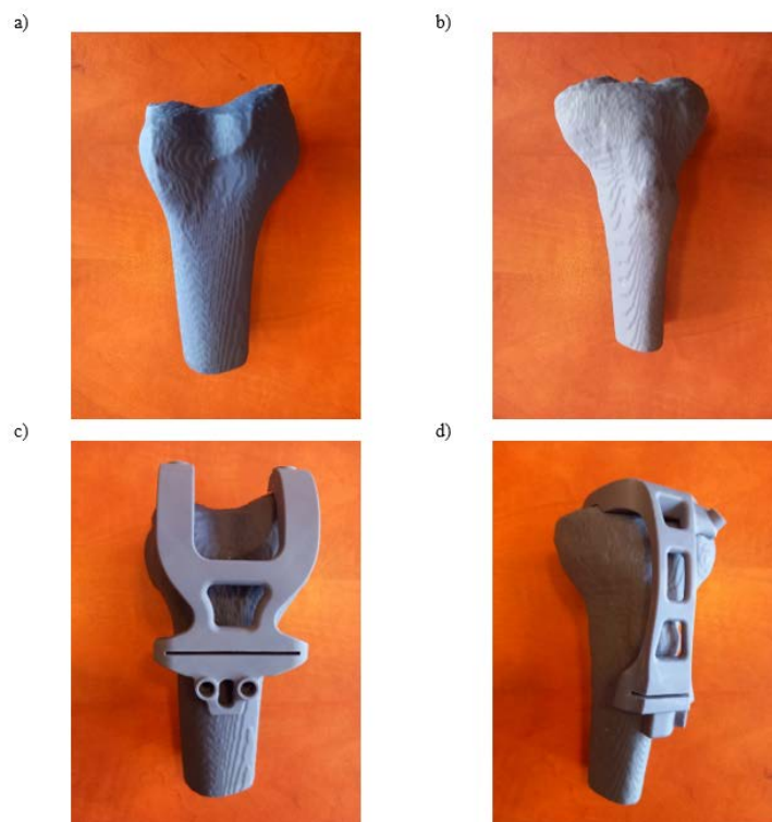
Figure 3. Rendered models: a) Femur bone; b) Tibial bone; c) Surgical guide for femur bone; d) Surgical guide for tibial bone
