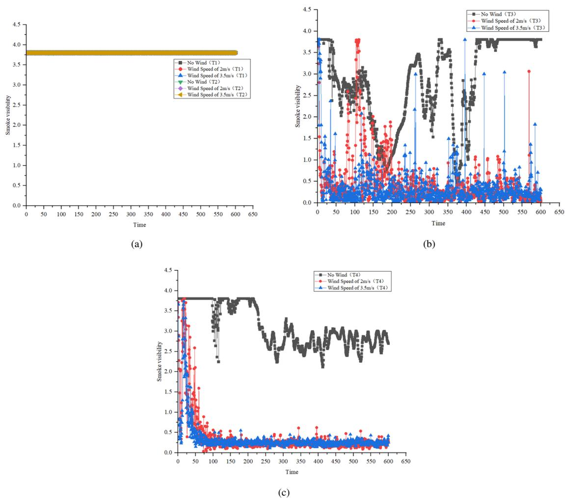
**Figure 11.** (a) Smoke visibility of T1 and T2 on the third floor; (b) T3 smoke visibility at different wind speeds on the third floor; (c) T4 smoke visibility at different wind speeds on the third floor
