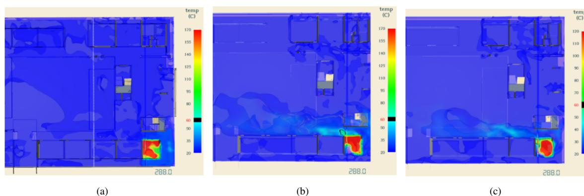
**Figure 13.** (a) No wind; (b) 2 m/s wind speed; (c) 3.5 m/s wind speed
