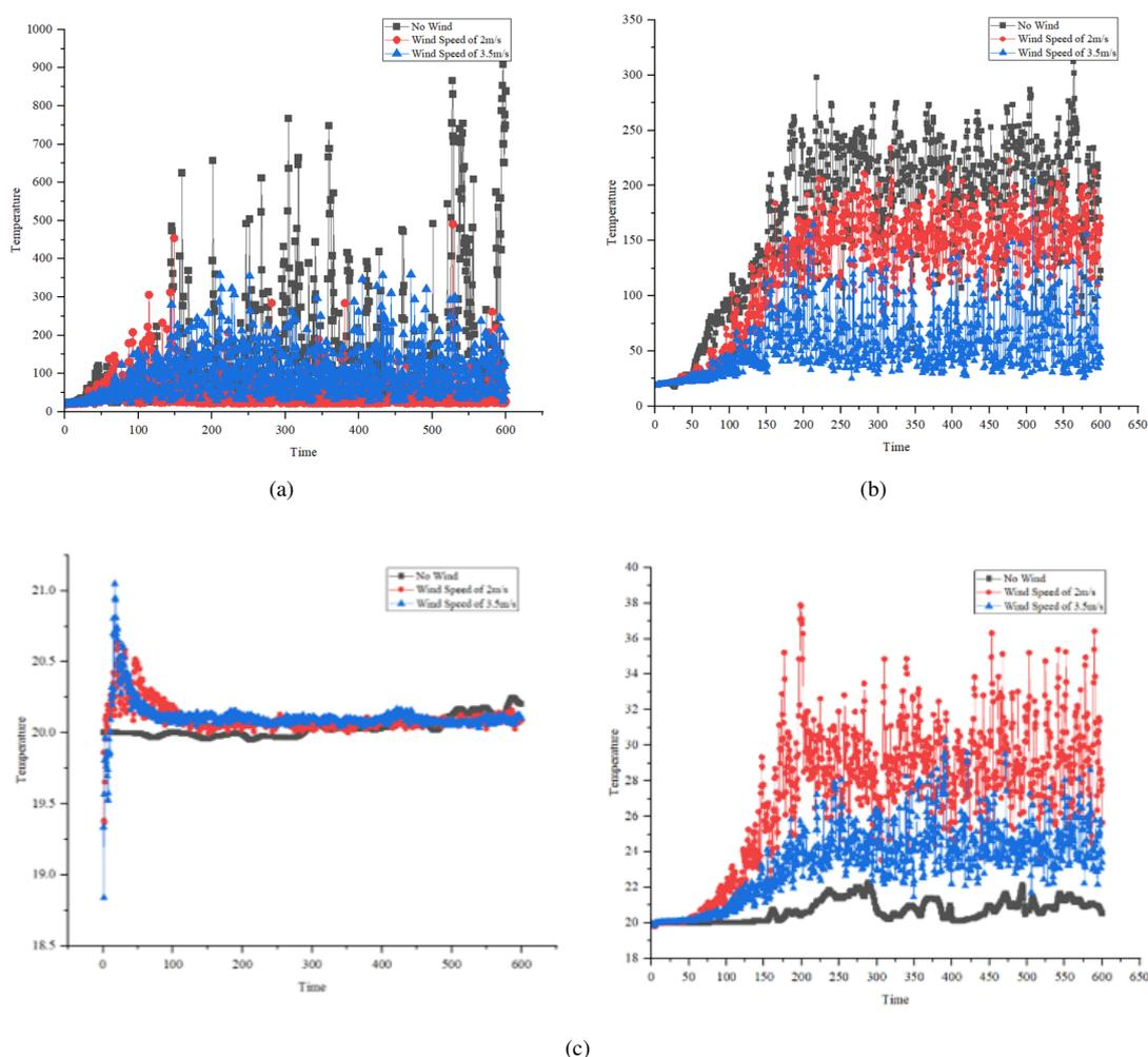
**Figure 12.** (a) Temperature variation chart of 1-D0 at different wind speeds on the first floor; (b) Temperature variation chart of 1-D00 at different wind speeds on the first floor; (c) Temperature changes of 1-D3 and 1-D4 at different wind speeds on the first floor
