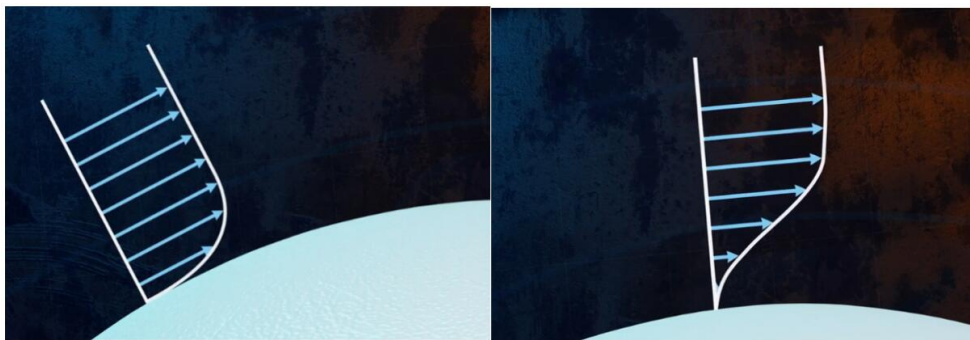
Figure 6. Pressure gradient changes on the train body surface under crosswind
