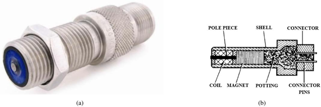
**Figure 1.** (a) VRS; (b) Main components of VRS [8]
