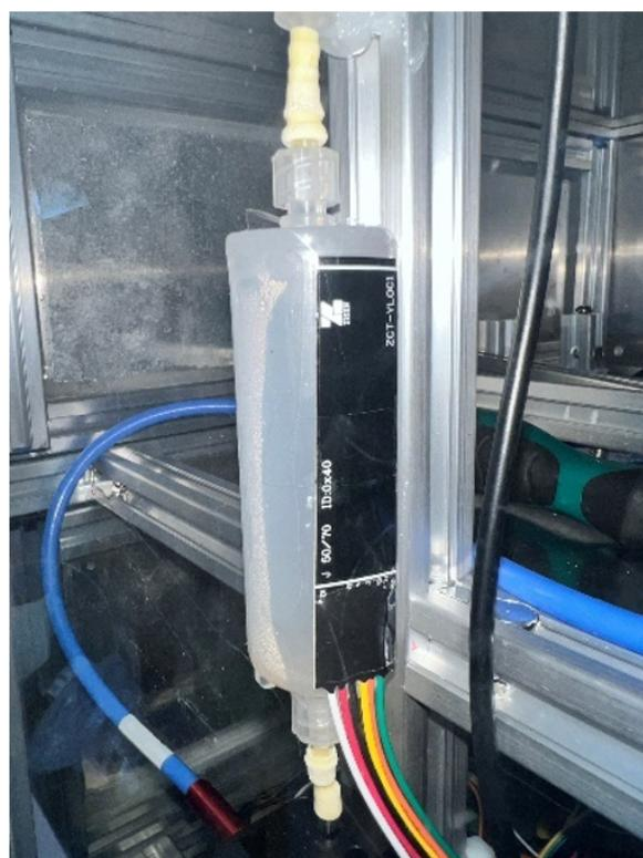
**Figure 1.** Physical view of the liquid buffer bottle and liquid level sensors
