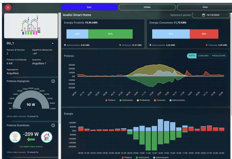
Figure 3. DHOMUS user interface: Real-time monitoring: Breakdown of energy into consumed, produced, withdrawn and fed into the grid, and self-consumed with different time references
