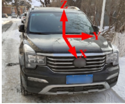
Figure 3. Schematic of automobile coordinate system
