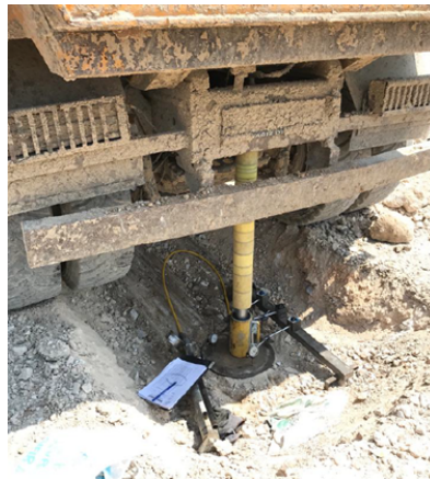
Figure 2. Plate load test setup
