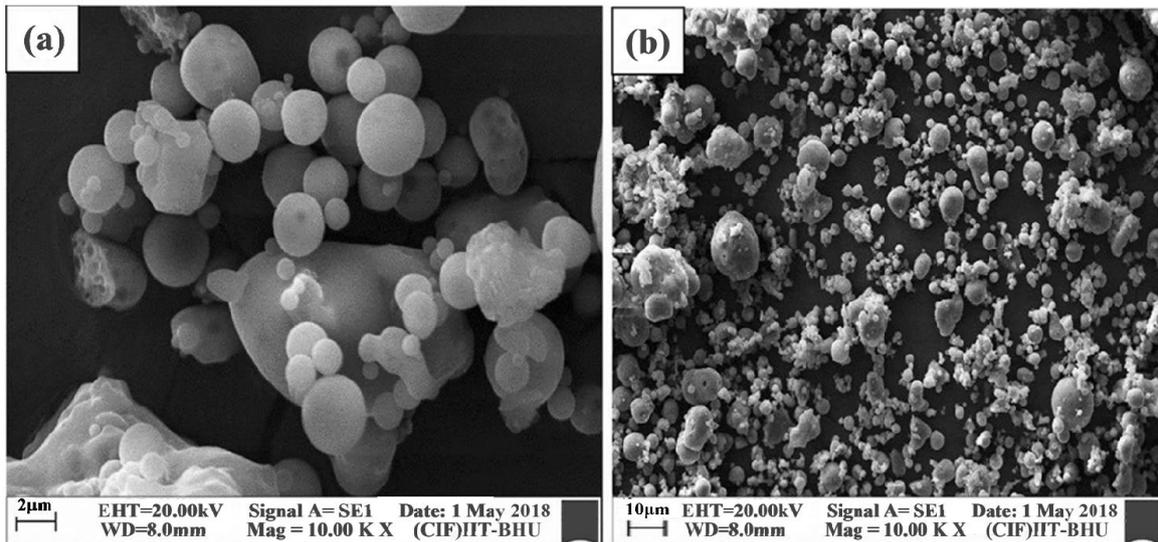
**Figure 5.** SEM analysis of MSW particle, a) 10.00Kx, b) 1.00Kx (Reddy et al., 2018)
