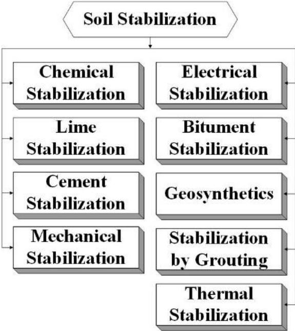
Figure 1. Different soil stabilization techniques
