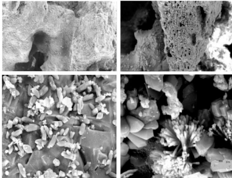
**Figure 3.** SEM images showing irregular shape of ash particles (Singh & Kumar, 2020)
