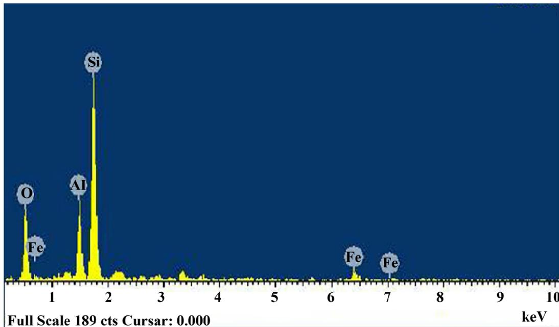
**Figure 6.** EDX diagram of MSW (Reddy et al., 2018)
