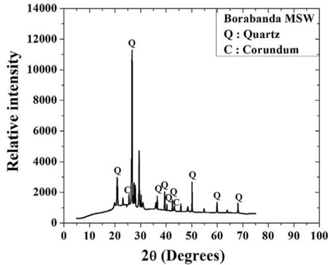
**Figure 4.** XRD pattern for MSWI ash (Reddy et al., 2018)
