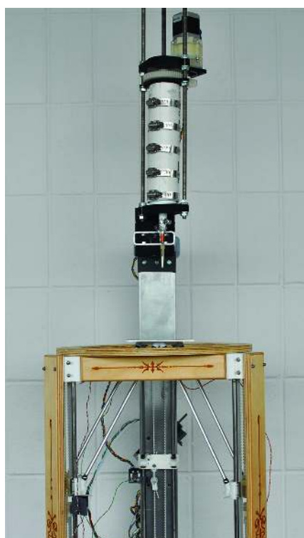
Figure 16. Upside-down delta 3-D printer with a stationary caulkstruder.
