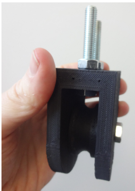
Figure 5. 3-D printable heavy-duty rope pulley.
