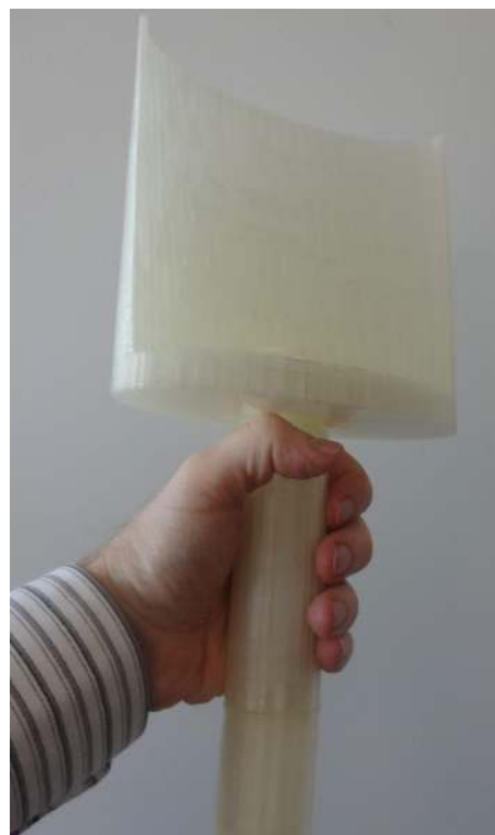
Figure 4. 3-D printable shovel with handle components that fit together to extend the reach to the necessary length.
