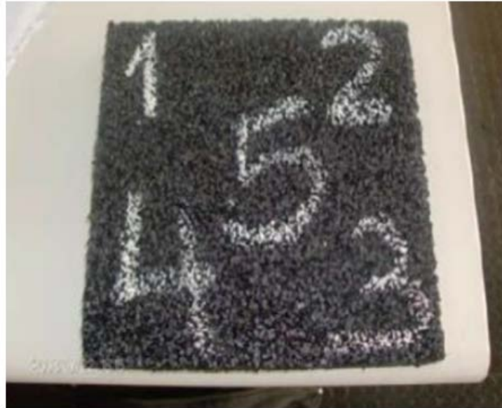
Figure 10. Example of a finished rubber agglomerate sample
