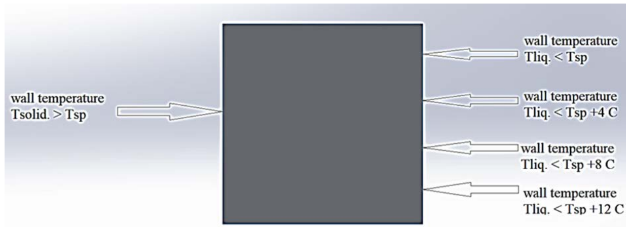
Figure 1. Division of the heat-supplying wall into four sections with varying temperature gradients
