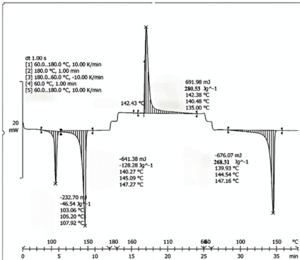
Figure 1. DSC curve of PCM 2
