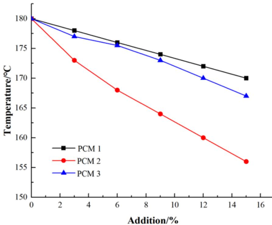
**Figure 5.** Experimental results of cooling performance for PCMs 1-3 in the drilling fluid
