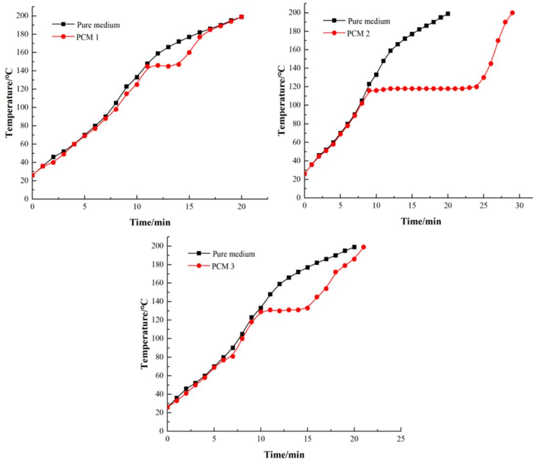
**Figure 2.** Heat storage and temperature regulation curves of PCMs 1-3
