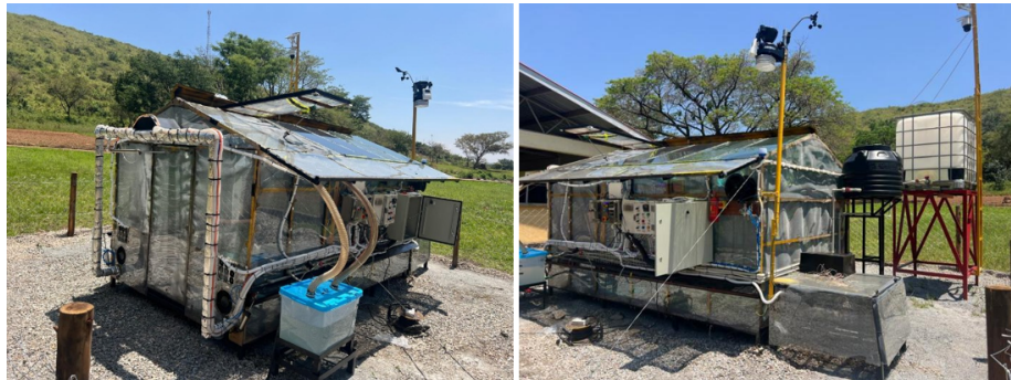
Figure 6. Fabricated smart integrated Cadmium Telluride (CdTe) greenhouse
