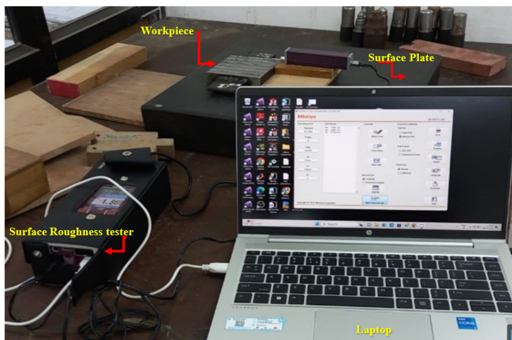
Figure 1. Surface roughness measurement of experimental workpiece
