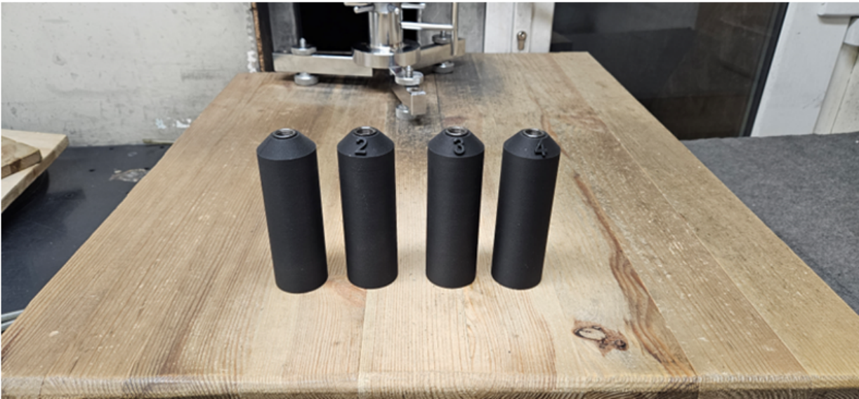
Figure 1. 4 non-typical suppressors for the .22 caliber rifle that are made with a 3D printer
