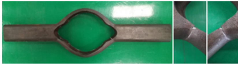
Figure 14. Cracking of the bridge shell and cracks
