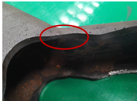
(b) Wall thickness reduction in the fragile zone
