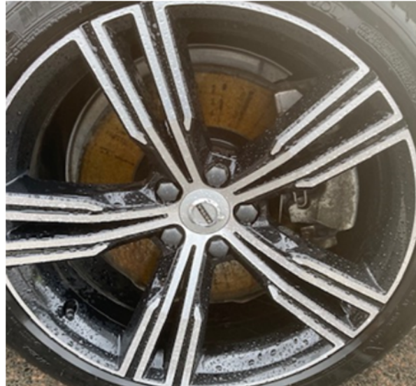
Figure 1. Rust development on the friction surface of untreated GCI brake disc mounted on a battery electric vehicle (BEV)
