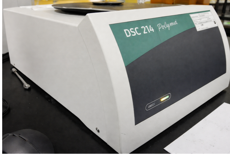
Figure 3. The differential scanning calorimetry (DSC) apparatus used for transformation temperature measurements
